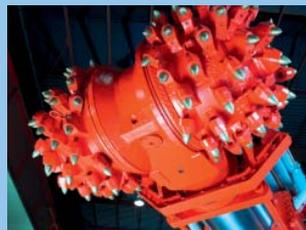
Cutter head of Tunneling roadheader MT720.
